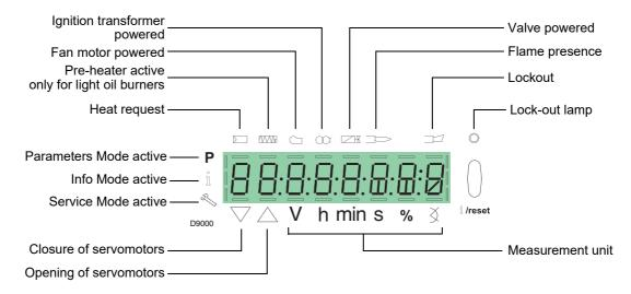
The display brightness can be regulated from 0 ... 100% with parameter 126.
