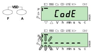
With the keys "+" and "-" select the first character of the password (letter or number), and confirm by pressing the key "i/reset".
