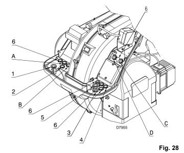
Cable grommets used in the factory:
