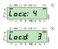
To reset, press the "i/reset" key for 1s: the display will show "rE-SEt". When the key is released, the lockout signal will disappear and the red indicator light will switch off. The control box is reset.
