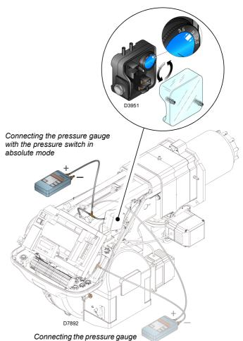
with the pressure switch in differential mode
