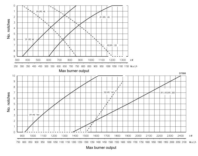
In the diagram (Fig. 19) find the notch at which to adjust both air and central gas/air.
