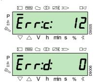
The burner goes into lockout.
