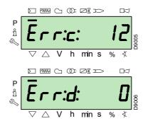
The burner goes into lockout.
