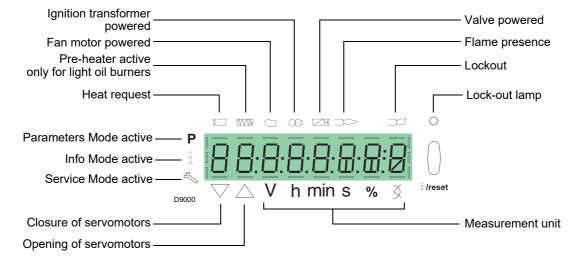
The display brightness can be regulated from 0 ... 100% with parameter 126.
