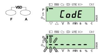
With the keys "+" and "-" select the first character of the password (letter or number), and confirm by pressing the key "i/reset".
