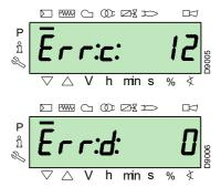
The burner goes into lockout.
