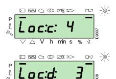
To reset, press the "i/reset" key for 1s: the display will show "rE-SEt". When the key is released, the lockout signal will disappear and the red indicator light will switch off.
