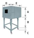
If noise emission needs reducing even further, sound-proofing boxes are available. When a lower "B" dimension is required, it is available the Box Support Kit code 20065135 which allows to reduce it at the fixed dimension of 55 mm. The sound-proofing boxes are not suitable for outdoor use.
