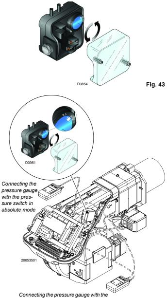
Connecting the pressure gauge with the pressure switch in differential mode
