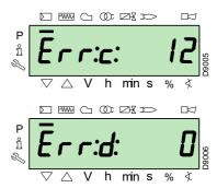
The burner goes into lockout.
